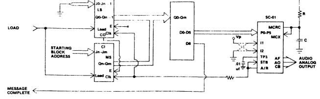
Figure 9. Multiple Message, Fixed Block Size
