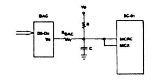
Figure 6. Variable Voice by Potentiometer Control
