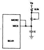
Figure 6. Variable Voice by Potentiometer Control
