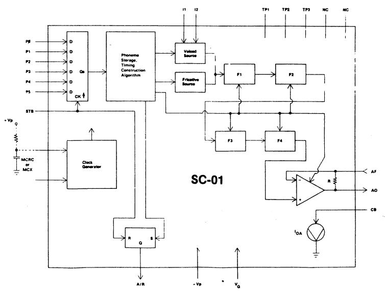
Figure 5. SC-01 Block Diagram
