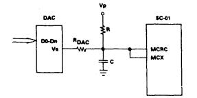
Figure 7. Variable Voice by DAC Current Injection
