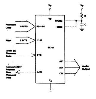
Figure 2. SC-01 Flow Diagram
